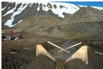
Figure 2. The waste rock pile with the drainage trench and the constructed weir used to quantify the discharge throughout the summer 2005. The trench was designed to collect all runoff coming from the pile. Daily measurements of element concentrations and continuously measured discharge made it possible to estimate the flux of dissolved weathering products from the pile.
